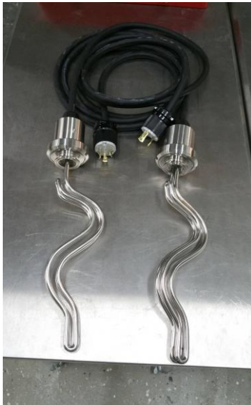
2 Stainless Steel Heating Element Assemblies: (1) short 8' (1) long 11'
